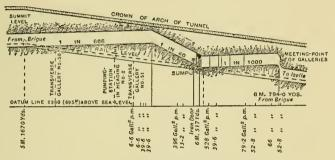
FIG. TO.—CHANGES OF GRADIENT ADOPTED IN DRIVING HEADING FROM BRIGUE BEYOND SUMMIT-LEVEL.
